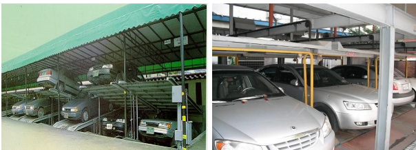
Fig. 5. Two-Stage Parking System
