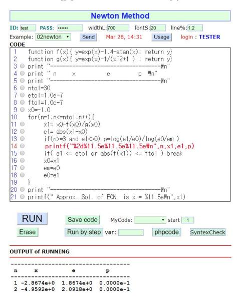
FIGURE 2. Step by Step Debugging Tool of NAPHP v2.0
