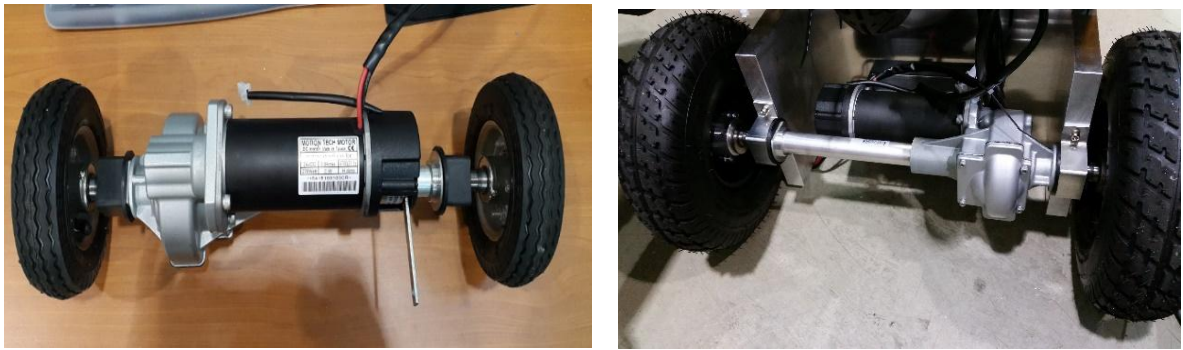
Figure 6. Manufactured rear systems applied trans-accel of a 3-wheel electric scooter
