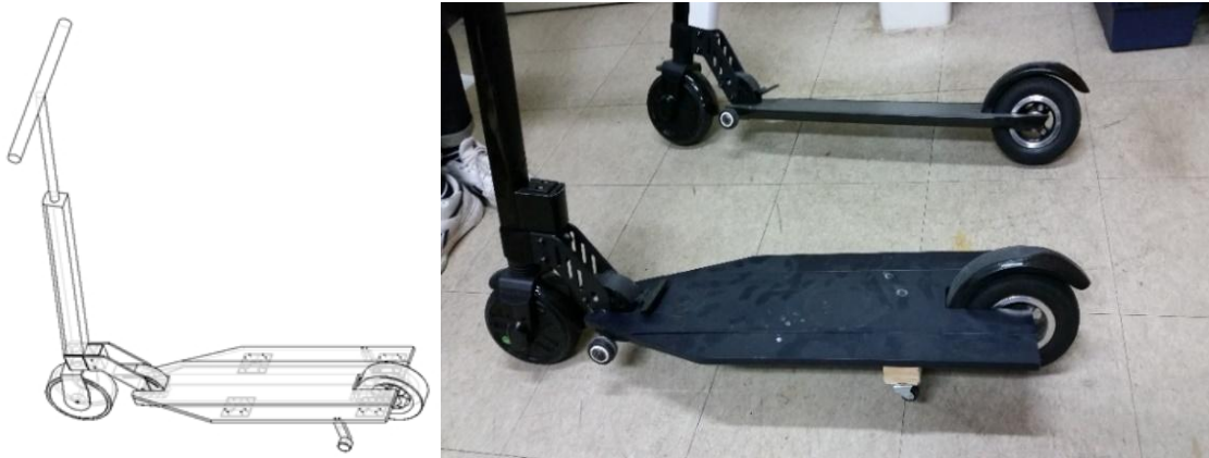
Figure 4. Prototype of a 2-wheel electric scooter equipped assist foot plate and caster
