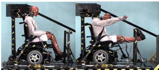
Fig. 1 Sled test of wheelchair occupant (7)
