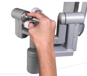
[Fig. 2] Master controller for da Vinci surgical robot
