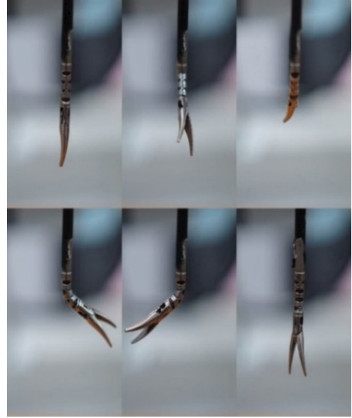
[Fig. 8] Control of da Vinci surgical tool
