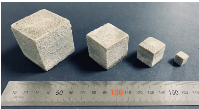
Photo 1 Binder Jetting 3D Printed Specimens after post-processing
