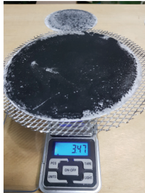
Fig 8 Sprayed Carbon (3.47g).
