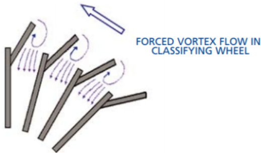
Fig. 2. Concept of forced vortex 7) .
