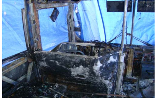
a) Fire producing example of driver seat right side
