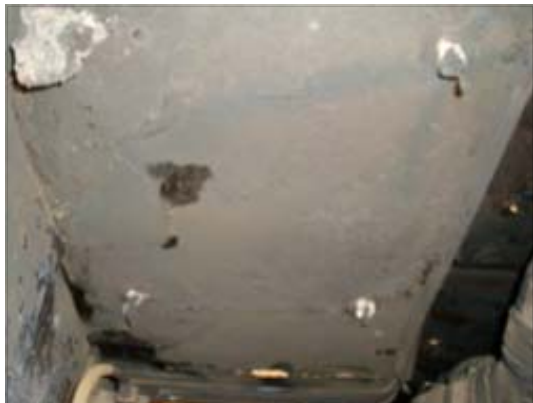
a) Acoustic absorbent material attached exhaust manifold upper part
