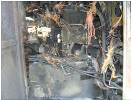
a) Fire example of CNG bus engine
