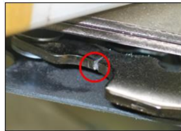
Fig. 4 Failure of hinge lever during endurance test of initial design
