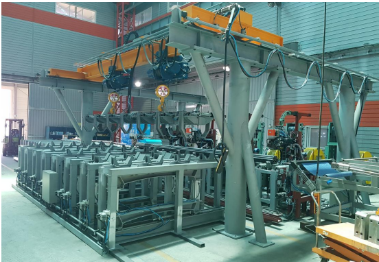
Fig. 10 Development of Cold Draw Bar Packaging Automation System
