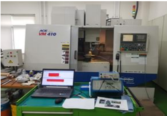
Fig. 3 Experiment setting of grinding force
