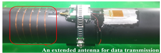
Fig. 11 An extended antenna for data transmission
