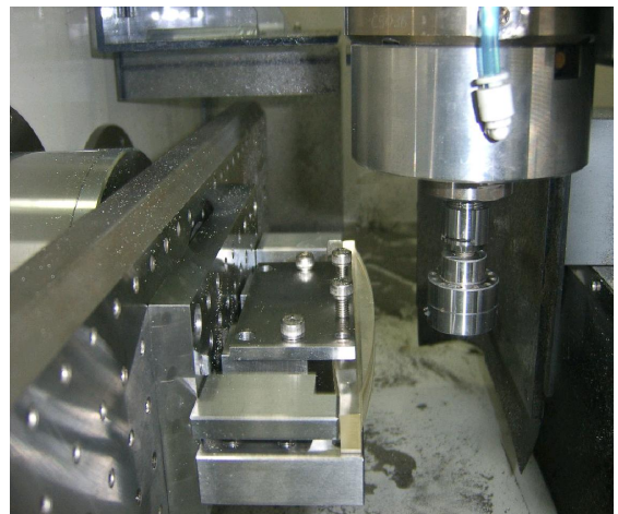
Fig. 6 Finishing process of master f-theta lens
