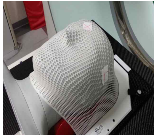
Fig.1. Anthropomorphic phantom setup for CT image acquisition.
