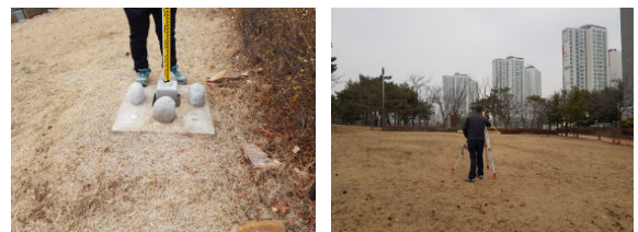
Fig. 6. Direct leveling from Unified Control Point, U08
