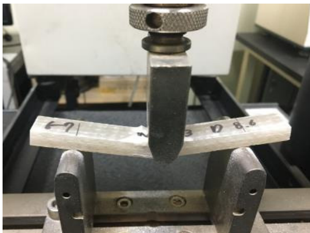
Fig. 2. Test for short-term flexural properties.
