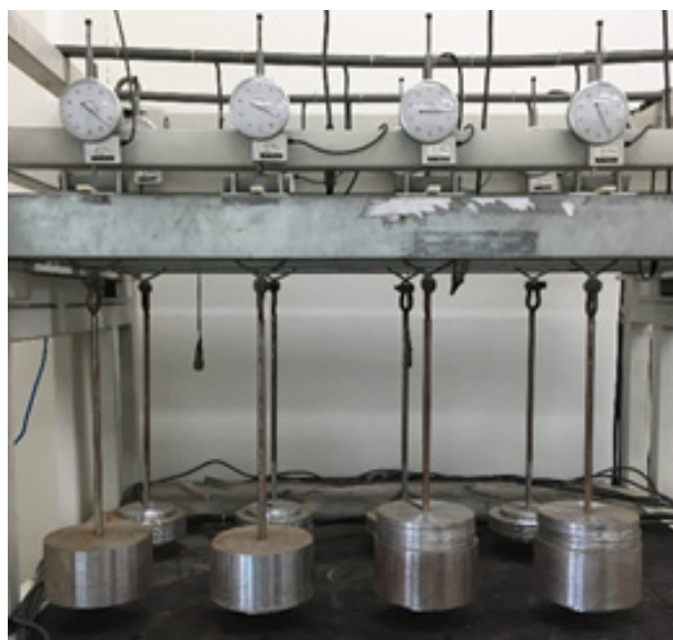
Fig. 4. Creep test loading.
