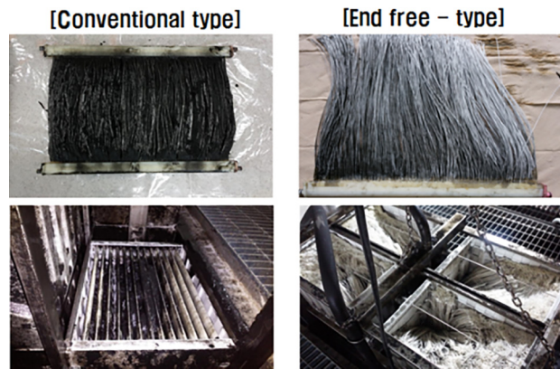
Fig. 10. Comparison sludge packing statue by membrane module type.
