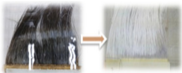
Fig. 15. Cleaning effect of Na 2 S 2 O 4 500 ppm by submerged method.
