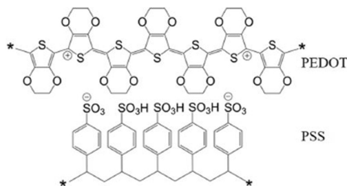
Fig. 1. Chemical structure of PEDOT:PSS (Tadesse et al., 2019).
