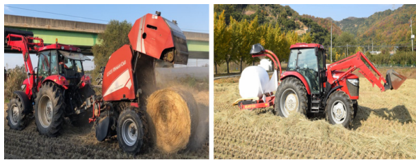
Fig. 5 Baler(left) and wrapping(right) operation for load measurement of tractor lifting pump
