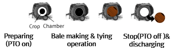
Fig. 7 Hydraulic pressure(up) and flow rate(bottom) of lifting pump and working procedure of round baler operation
