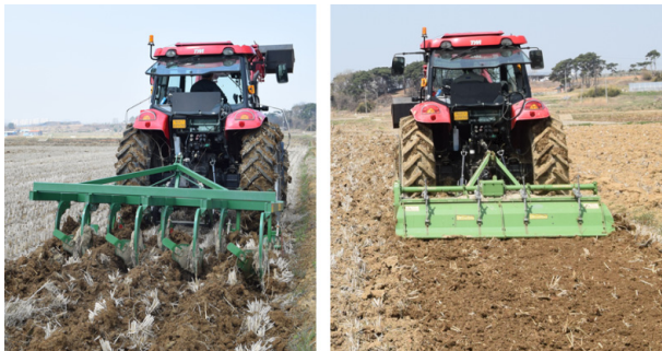
Fig. 1 Plow(left) and rotary(right) tillage for load measurement of tractor lifting pump
