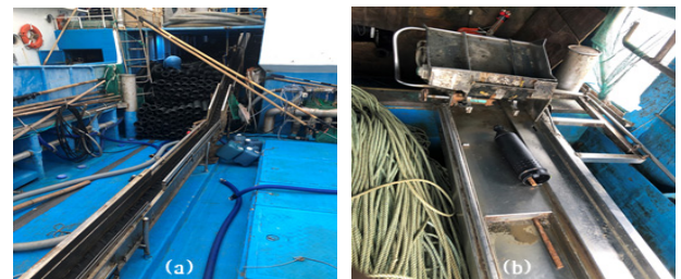
Fig. 4. The status of fishing equipments and fishing system in the offshore conger eel pot fishery. (a) carrying and loading devices, (b) casting devices.
