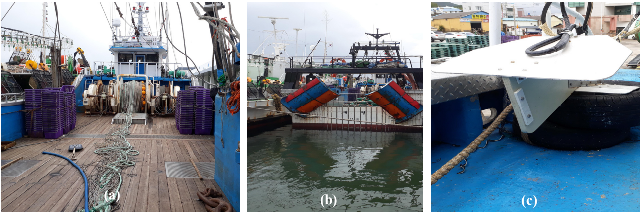
Fig. 3. Net drum, trawl winch (a), otter board (b) and net recorder receiver (c) etc. fishing equipments on the deck of Eastern Sea trawl vessel.
