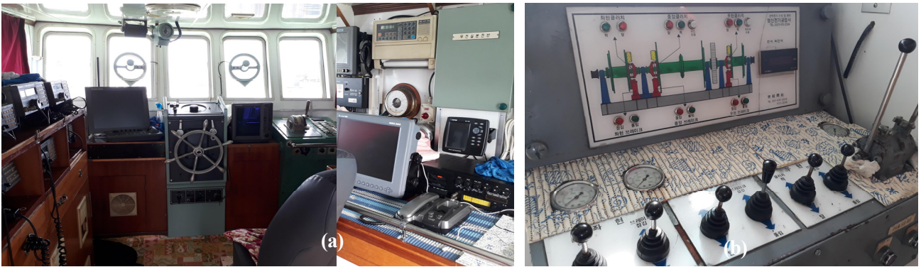
Fig. 2. Navigation systems (a) and winch controller (b) in the bridge of Eastern Sea trawl vessel.
