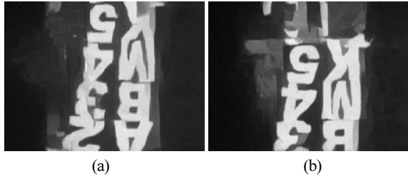
[Fig. 7] Generated images from the neural network. Sonar images are converted as optic style image
