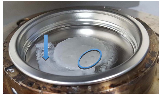
Fig. 4. Error factors of the polymerized nylon 6 after measuring viscosity (reaction temperature : 150°C)
