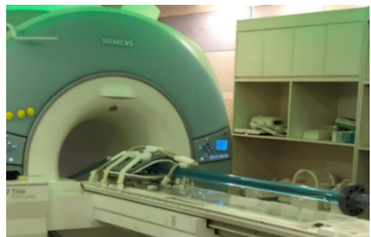
Fig. 4. 3T MRI machine and pipe test section (with RF torso coil)
