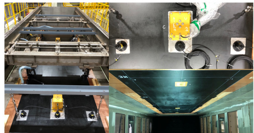
Fig. 10. Installation of sensors at flat plate (B×L : 1.2m×4.8m) inside large cavitation tunnel
