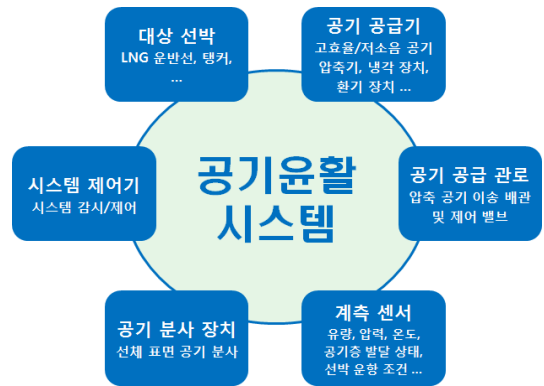
Fig. 2. Main components of air lubrication system
