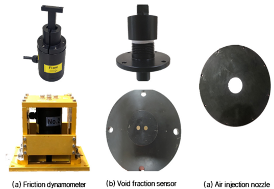
Fig. 6. Measuring sensors & Air injection nozzle
