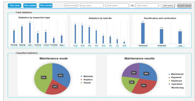
Fig. 13 Tank Inspection Finding Problem Statistics Analysis Page.
