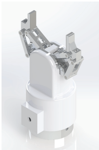
Fig. 6 3D modeling of the adaptive gripper with actuation type I
