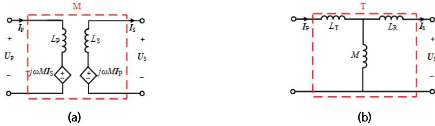
Fig. 3 Equivalent models of loosely coupled transformer. (a) M model. (b) T model.
