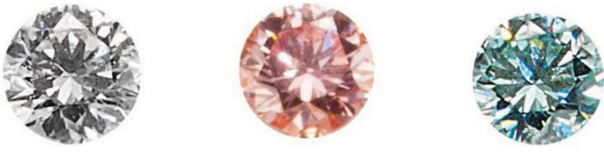
Fig. 1. Three Lightbox CVD grown diamonds. These near colorless 0.25 ct (left), Fancy Vivid orangy pink 0.25 ct (middle) and Fancy Vivid blue 0.26 ct (right) samples were recently examined by Hanmi Laboratory.
