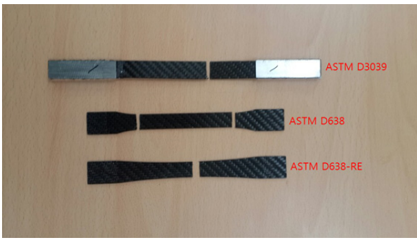
Fig. 9 Photograph showing representative rupture locations
