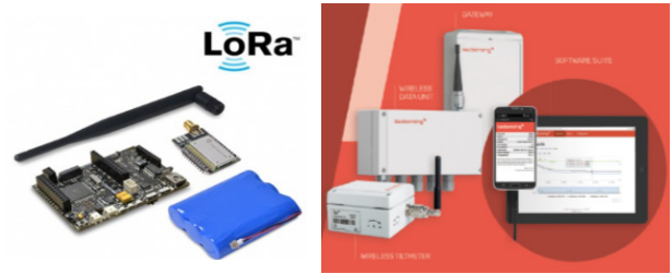
(a) LoRa IoT equipment (b) Wireless tilt measurement system
