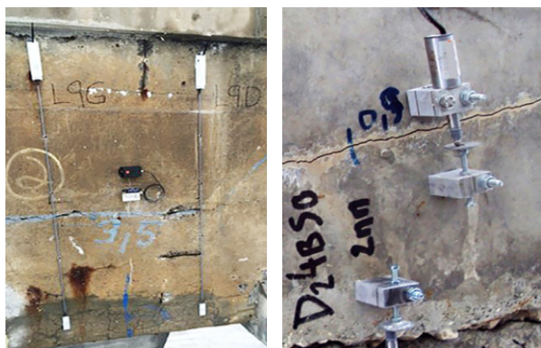
Fig. 6 LoRa based wireless sensor application case(turcot intersection in canada)
