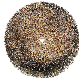
Fig. 6. Combustion catalyst after end of experiment
