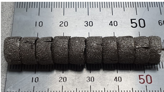
Fig. 2. Nickel foam cup for holding catalyst in multilayer cup structure (MLCS)
