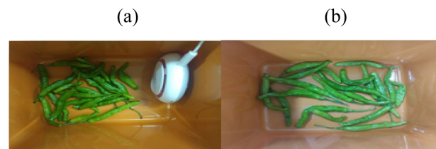
Fig. 1. Photos of the test to determine the effect for the reduction of microorganism on hot pepper by a commercialized plasma device. (a) Hot peppers and plasma device, (b) Hot peppers only.
