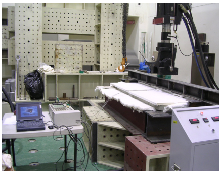
Fig. 2. Set up of specimen on electric furnace with glass wool
