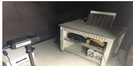
Fig. 3 Thermal image measurement of large area carbon planar heating elements
