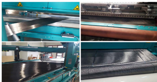
Fig. 6. Carbon NCF Fabric manufacturing process
