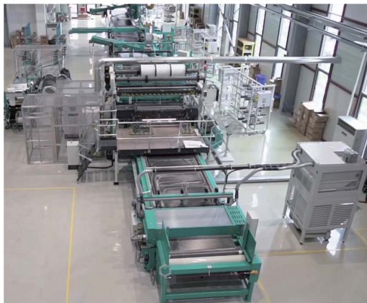
Fig. 3. Multi axial carbon fabric weaving machine(NCF)
