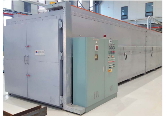
Fig. 4. Thermoforming system of CFRP with multi function (oven)
