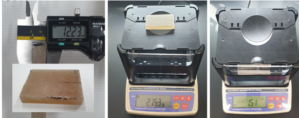
Fig. 4 Measurement of the relative densities from sample GFRP using a hydrometer
