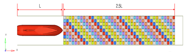
Fig. 6 Finite element model for towing simulation of a research icebreaker
