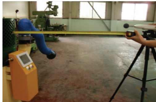
Fig. 7 Sound pressure level test
