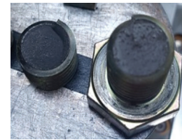
Fig. 2 Appearance of failure bolt
