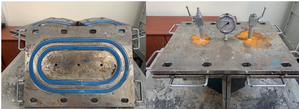
Fig. 3. Test apparatus for hydrophilic rubber waterstop (2 layer)
