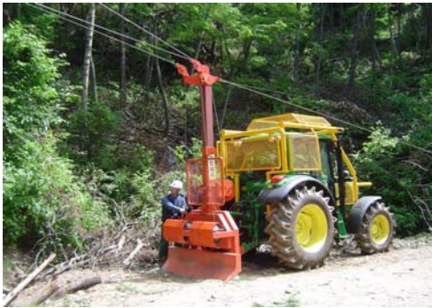
Fig. 4. Tower-yarder attached tractor and tower-yarder made in Korea.
