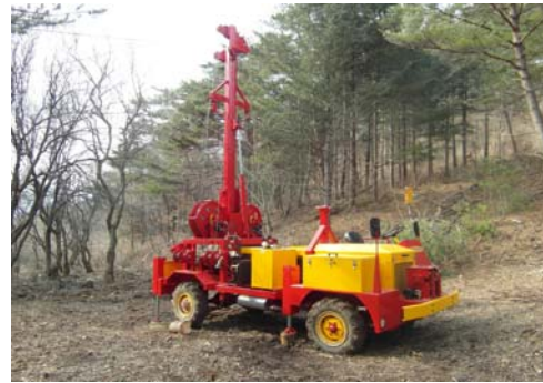
Fig. 4. Tower-yarder attached tractor and tower-yarder made in Korea.
