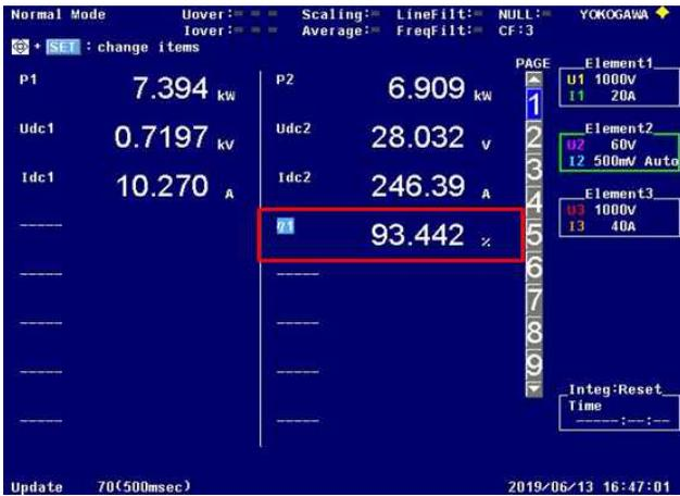
Fig. 15. Measured efficiency at rated input voltage and 7kW full load.
