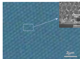
Fig. 6. Nano pattern image for nano frame by optical microscope and scanning electron microscopy.
