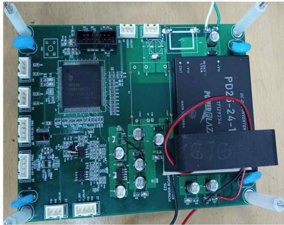
Fig. 11. Control system of the proposed converter based on TMS320F28377S.
