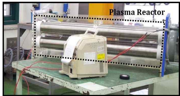
Fig. 12. The picture of plasma reactor for gas treatment.
