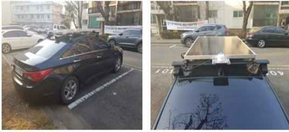
Fig. 1. Test vehicle with a photovoltaic module.
