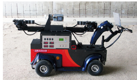
Fig. 3. Three-Dimensional Inspection Robot (ARGOS)
